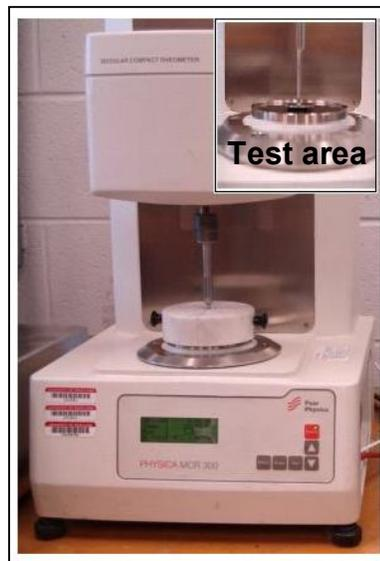
Figure 2.2. Paar Physica MCR 300 parallel disk rheometer
