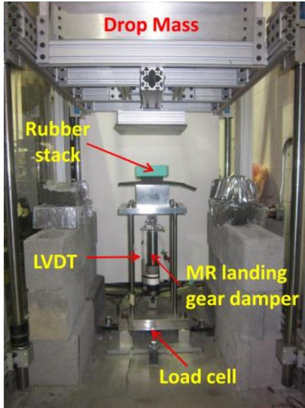
Figure 5.1. Single MR landing gear damper drop test setup at the University of Maryland
