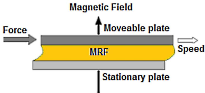
Figure 1.10. MR damper mode of operation: shear mode
