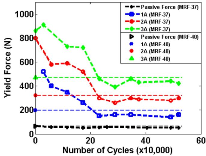
Figure 3.9. MR damper yield force as a function of number of cycles
