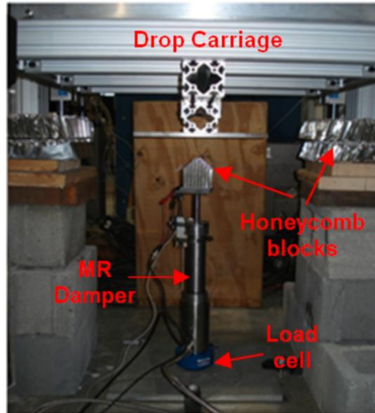
Figure 2.11. MREA drop testing setup at the University of Maryland
