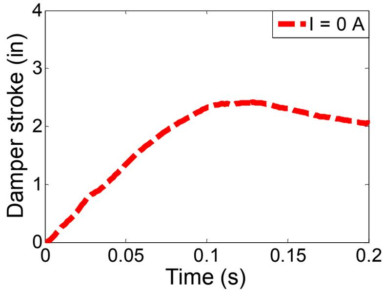
Figure 6.7. Transient piston displacement response measured with an LVDT at a nominal drop speed of 6 ft/s (1.8 m/s)
