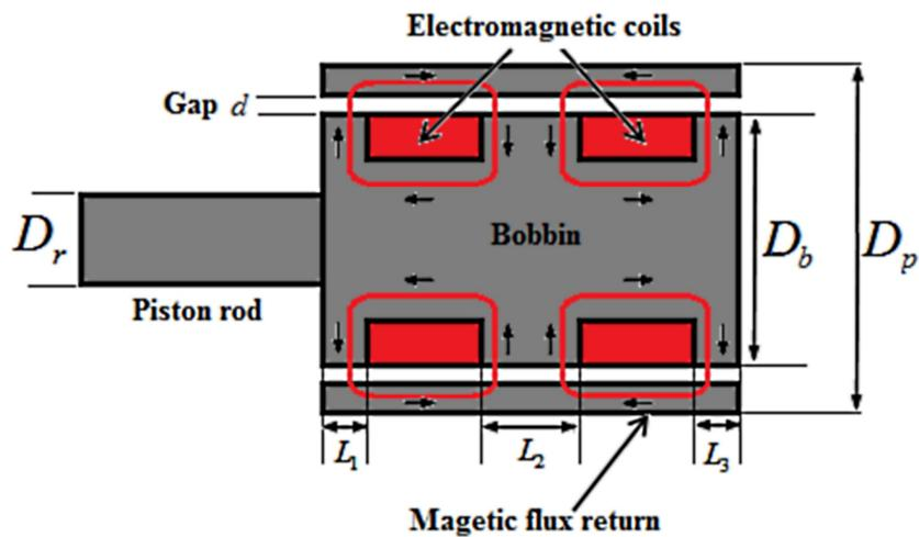
Figure 1.4. Typical conventional MR damper valve configuration
