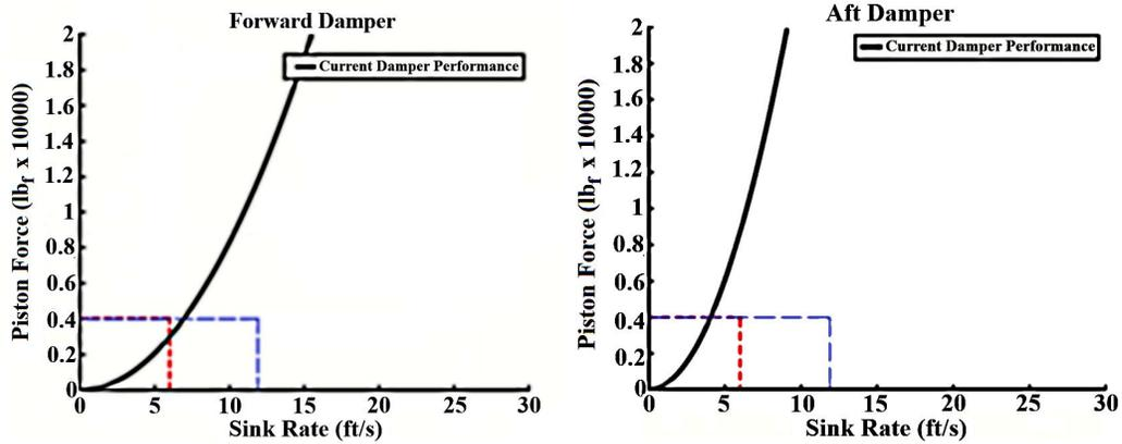
Figure 1.2. Passive hydraulic damper performances for the MD-500 helicopter fixed landing gear dampers. Each damper is tuned for only one condition.
