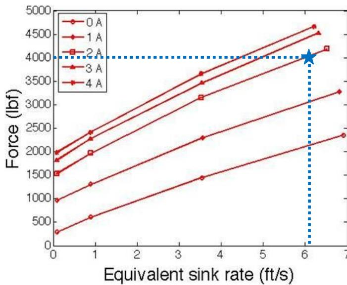
Figure 4.20. MTS machine capability of reaching equivalent sink rates of about 6.2 ft/s (or 1.89 m/s) while maintaining a stroking load of 4000 lb<sub>f</sub> in the landing gear damper at the University of Maryland
