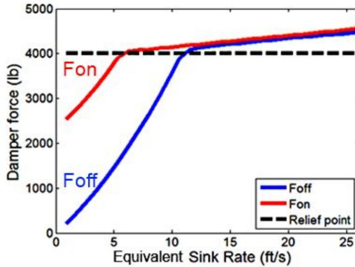
Figure 6.3. Predicted damper force of the relief valve of the MR landing gear damper versus sink rate with a desired spring stiffness of 50 lb<sub>f</sub>/in (8.76 kN/m)
