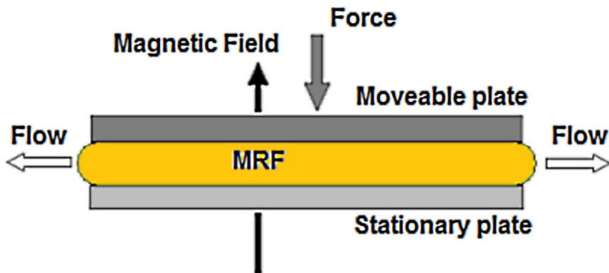
Figure 1.11. MR damper mode of operation: squeeze mode
