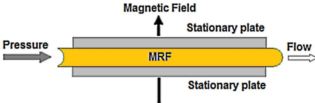
Figure 1.9. MR damper mode of operation: flow mode
