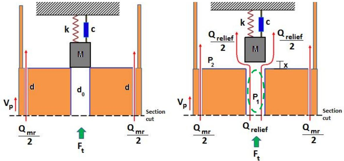
Figure 6.13. Hydraulic model of the MR and passive valves of the MR landing gear damper: (a) relief valve is closed; (b) relief valve is open and the pressure  $P_1$  across the center orifice is considered
