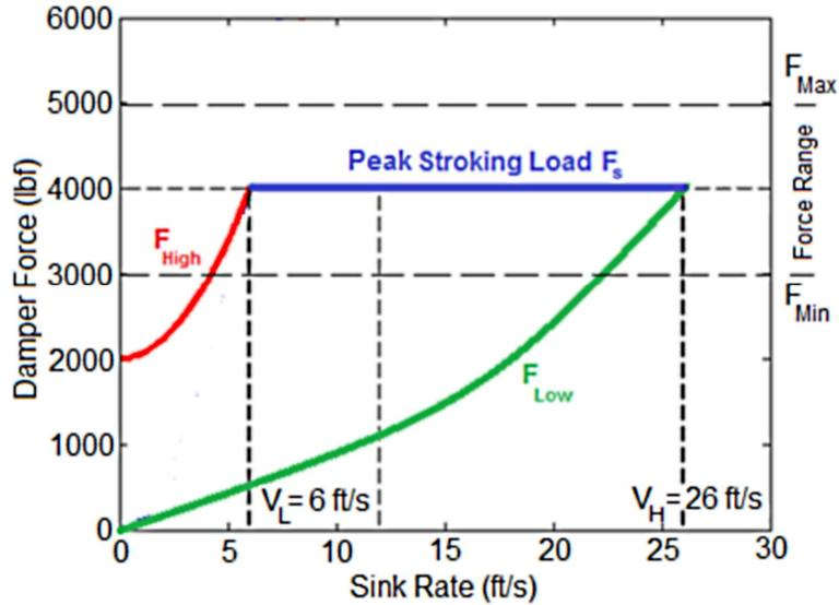
Figure 1.1. Design targets assigned by Boeing to maintain a constant stroking load of 4000  $lb_f$  over an equivalent sink rate range of 6-26 ft/s
